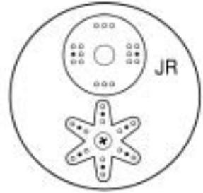
Mount the Steel Link Ball at 10.5mm (approx 7/16") from the center of the servo horn for the throttle arm.
